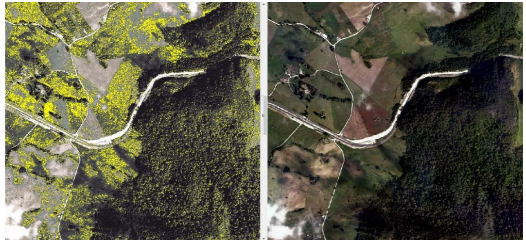
The image on the left shows the unsupervised generalization, including shadows of clouds. The image on the right is the original mosaic.
